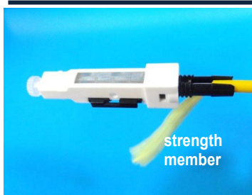
6. Insert fiber to QSC until it touches the fiber inside.
